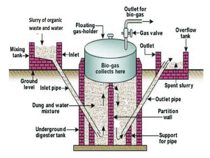
Bio-methanation is a process by which organic waste is microbiologically converted under anaerobic conditions to biogas. It is the most energy efficient and eco-friendly method for treatment
